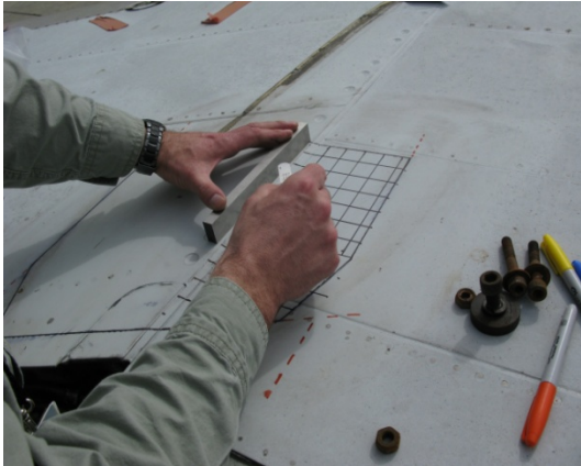
Step 1: Grid out doubler profile using 1 inch x 1 inch squares.
