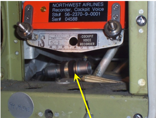
SLS connector routed to access panel
