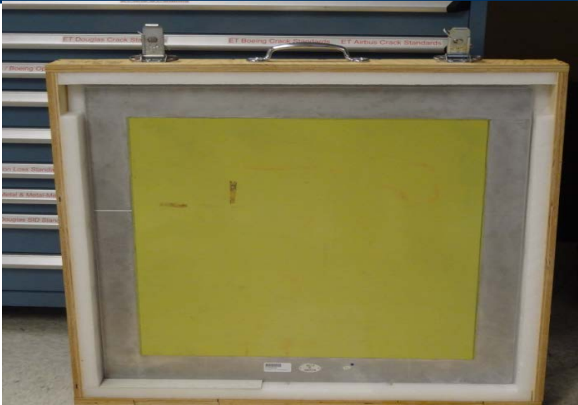
Honeycomb sandwich bonded to aluminum backing - calibration standard for body area bond test inspection
