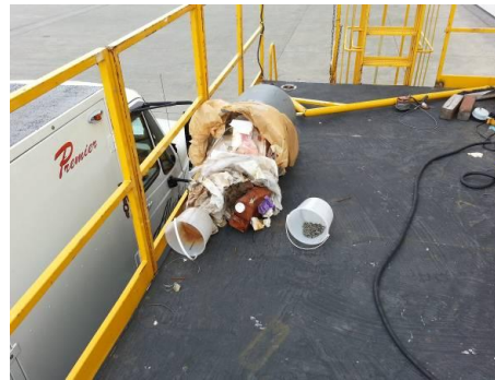
Figure 5 – Unsecured material (garbage) on platform
