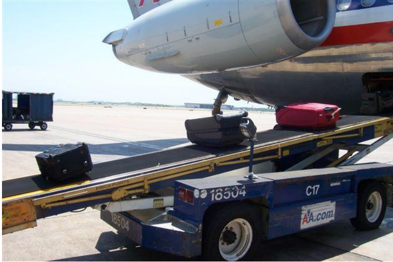
Figure 2 - Correct baggage spacing for loading and unloading
