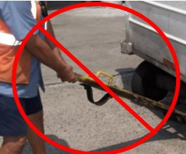
• Raise the tongue with an open hand on the bottom of the connection ring when putting tongue in the stowed position
